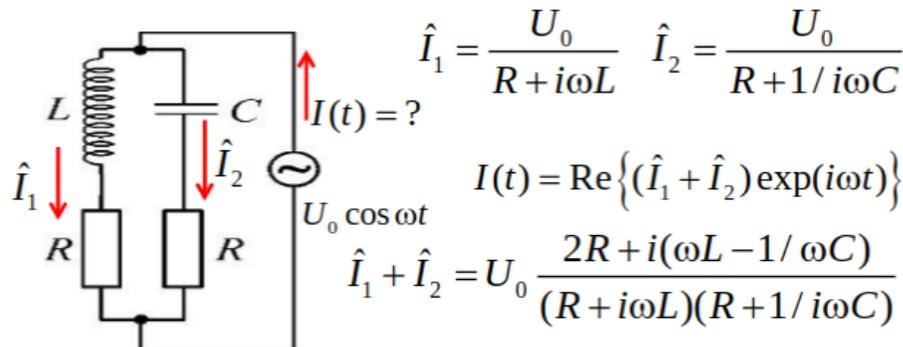
$$I(t) = U_0 \frac{\sqrt{4R^2 + (\omega L - 1/\omega C)^2}}{\sqrt{(R^2 + L/C)^2 + R^2(\omega L - 1/\omega C)^2}} \times \cos\left\{\omega t - \arctg(\omega L/R) + \arctg(1/\omega RC) + \arctg\left(\frac{\omega L - 1/\omega C}{2R}\right)\right\}$$
